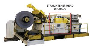
**Viking Inc.** – After a factory fire, much of the equipment was inoperable due to smoke and water damage from their fire protection system. This included two COE Press Equipment servo roll feeds installed in 2007 with control panels that were left in standing water. Through power washing, full mechanical rebuilds and new electrical systems with ServoMaster Touch Controller upgrades, both machines were brought to 'like-new' standards.
