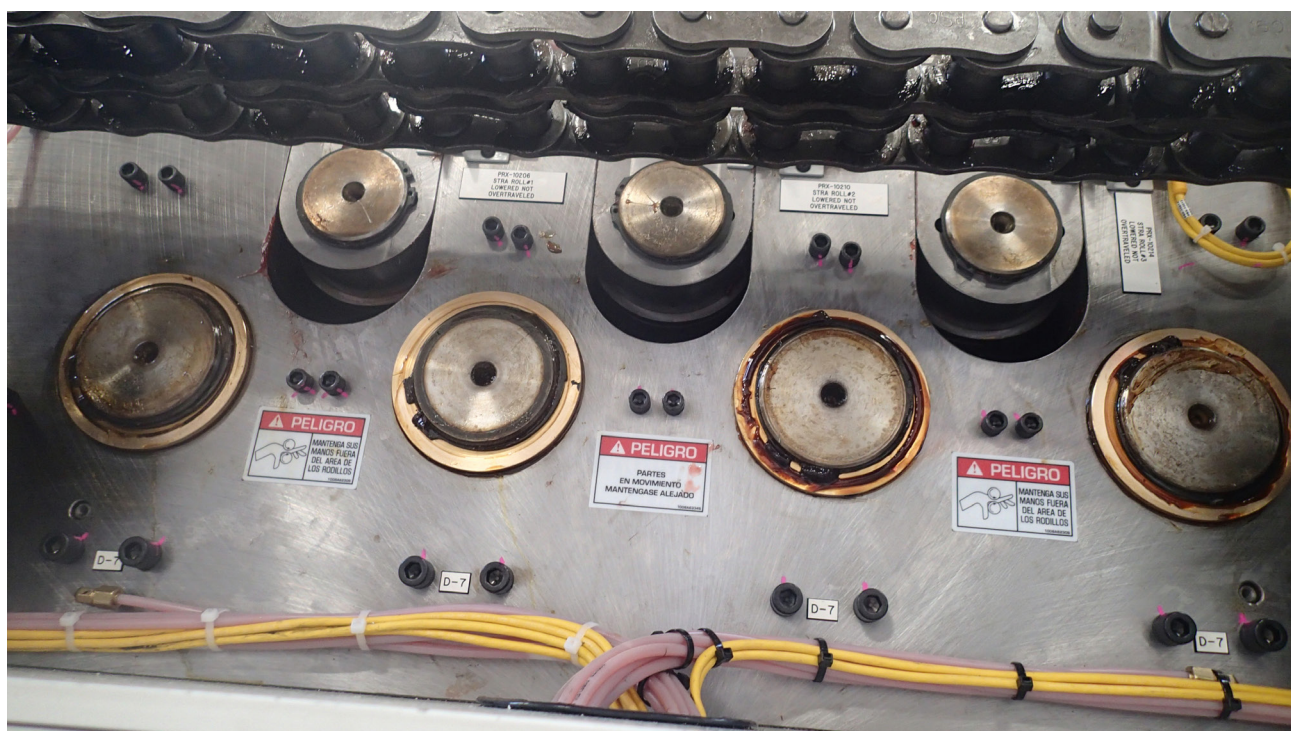
Processing of AHSS requires increased roll depth penetration.
